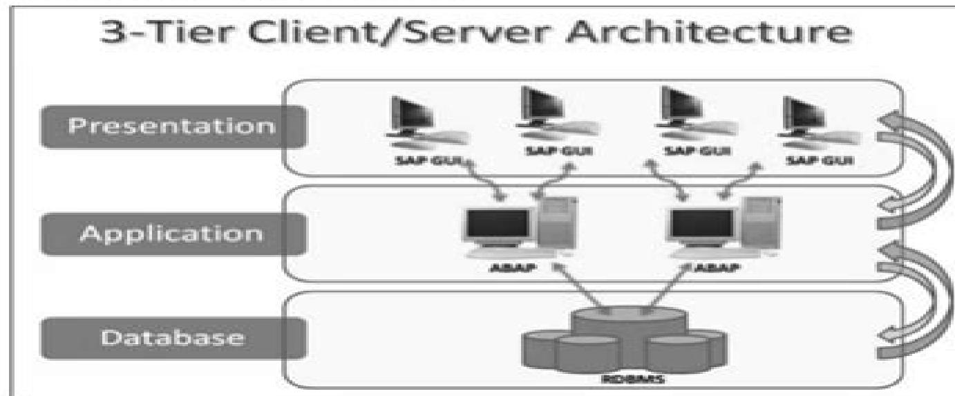
The **Presentation layer** consists of any input device that can be used to control SAP system. This could be a web browser, a mobile device and so on. All the central processing takes place in **Application server**. The Application server is not just one system in itself, but it can be multiple instances of the processing system. The server communicates with the **Database layer** that is usually kept on a separate server, mainly for performance reasons and also for security.
