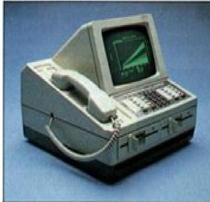
tached to the CBX system to communicate with the outside world. The system includes 512K bytes of memory, two 5 1/4-inch disk drives, a 9-inch monitor, and MS-DOS 2.11.
