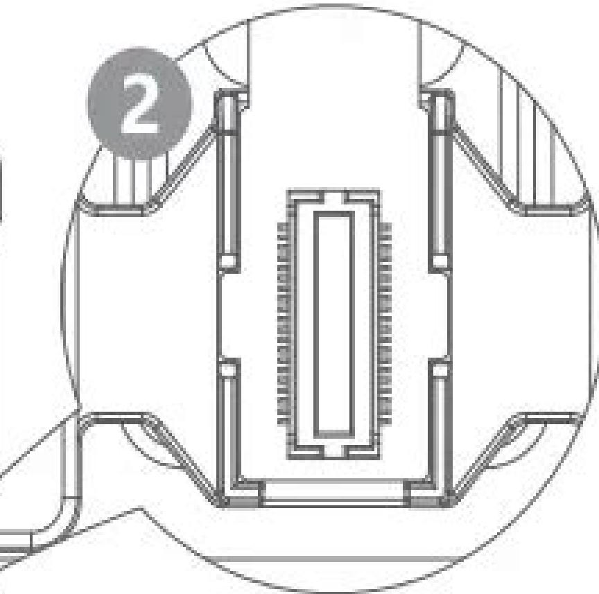
Attention: Insert the sub-unit interface into the groove on the magnetic stand as shown in the picture.
