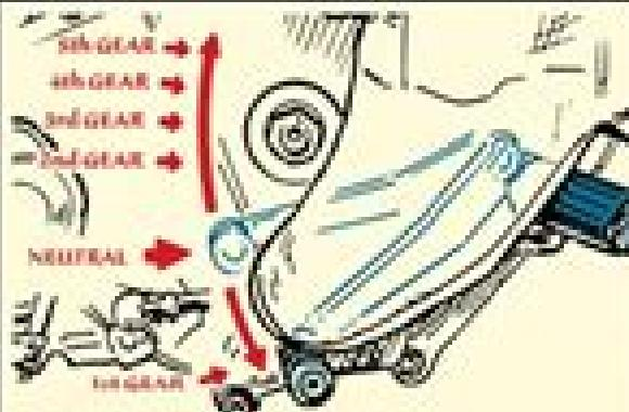
5. Shift to higher gears by pulling up on the gear shift with your foot. To shift down, push the gear shift down. Neutral is located halfway between 1st and 2nd gears—press lightly up from 1st gear or lightly down from 2nd.
