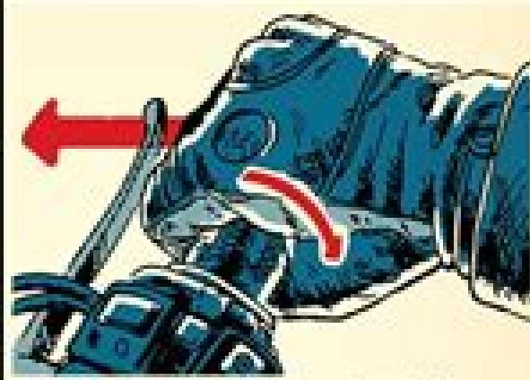
3. Slowly release the clutch lever until you start to feel the motorcycle pull. As it pulls, twist the throttle slightly to increase the engine's RPMs.
