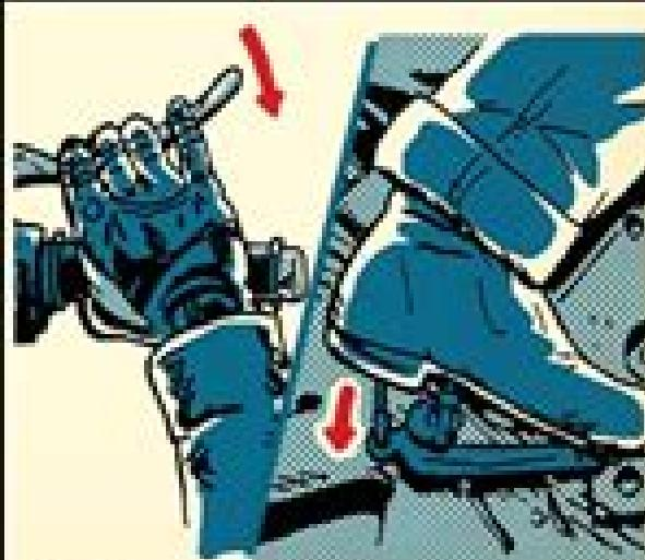
6. Bring yourself to a stop by using the front and rear brakes in tandem.
