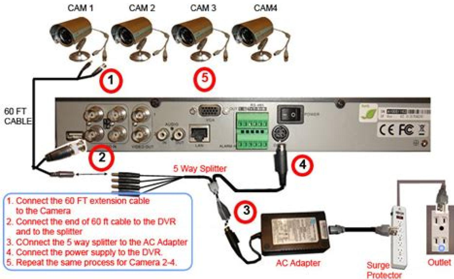
Notice: We STRONGLY recommend that you plug the DVR and Cameras into a Transient Voltage Surge Protector (UL-1449 rating). Look for a clamping voltage of 330 or lower, Joule rating of at least 400, and a response time of 10 nanoseconds or less.
